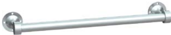
0755-SS HEAVY DUTY STAINLESS STEEL TOWEL BAR Towel bar fabricated of 1" (25 mm) O.D. x 20 gauge, type 304 stainless steel with a #4 satin finish and designed not to turn in support posts. Support posts fabricated of heavy brass with satin finish to match stainless steel. Available in 18", 24", 30" and 36" (460, 610, 760 and 915 mm) lengths.
