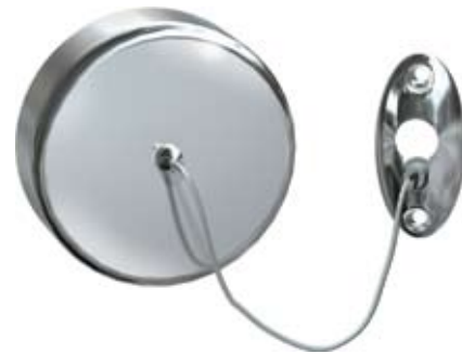
0712 SURFACE MOUNTED RETRACTABLE CLOTHES LINE Polished stainless steel unit has spring actuated 6 foot (150 mm) vinyl cord with white vinyl knob and locking nut to hold stretched line taut. Installs over bathtub or in shower.
