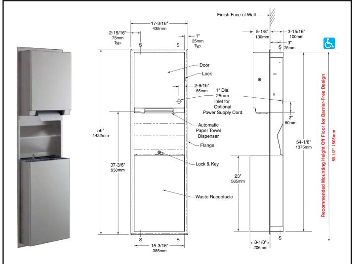
Rough Wall Opening 16" (405mm) wide 54-3/4" (1390mm) high 4" (102mm) minimum recessed depth
