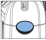
Lift latch to remove front cover. See dust bag for replacement instuctions.
