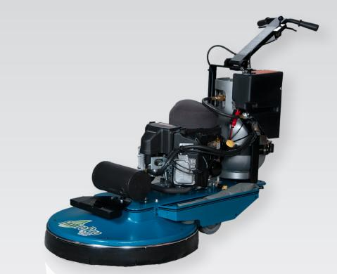
**The EnviroPro Series** increases floor temperature during burnishing so that the gloss level rises with use of densifers. Built to meet GS-40 and LEED standards set for floor maintenance to capture dust and keep the working environment safe. This aluminum frame burnisher controls airborne debris with a unique air funnel system that traps and filters dust. Run time is 5 to 6 hours for one propane cylinder.
