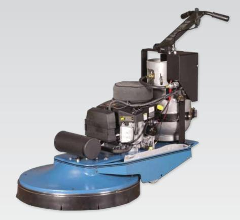
The Dust Control Series provides a variety of buffing widths in a high powered propane machine. Available with your choice of Kawasaki or Robin engine. Run time is 5 to 6 hours for one propane cylinder. Emissions protected by 3-way catalytic muffler.
