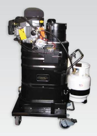
SK300 is a propane powered vacuum that works great at removing fine dust particulates like concrete dust. This 300 CFM propane powered vacuum is just the right size for two walk behind grinders. Matched perfectly to the task of dust control for a G & P ONE, this 17 Hp machine will run up to 6 hrs on a tank of propane. Carbon impregnated, anti-static housing with manual shaker.
