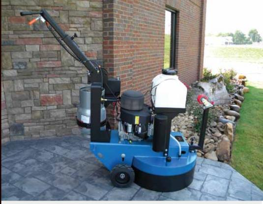
The LX – 30 Propane Powered Grinder and Polisher. It utilizes three 13" counter rotating heads, with either 9 or 12 diamond discs. A hefty 700 lb. of concrete grinding muscle, taking concrete surface prep, grinding and polishing to new levels.
