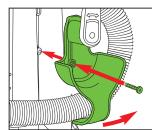
Attach hose retainer with one short screw. Pull retainer out to position hose.
