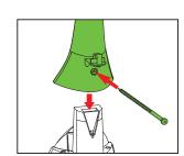
Slide handle onto tool caddy. Fasten with one long screw.
