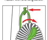
Push cord into upper cord retainer. Place hose over hose hook on handle.
