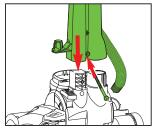
Slide vacuum back onto base. Fasten with one long screw.
