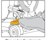
Step on handle release to lower handle into position.
