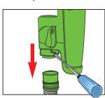
Some models: Secure bottom of duster chamber to hose retainer. Tighten with flat-head screwdriver.
