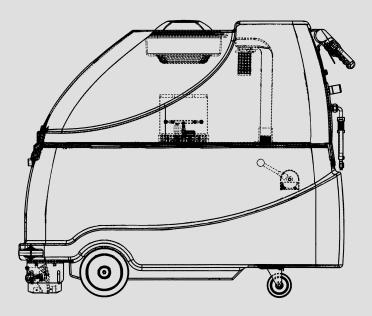
The Paramount automatic extractor has a 40 gallon recycling tank. Combine that with the CFR recycling chemical technology and the Paramount produces a cleaning solution volume capacity up to 240 gallons.
