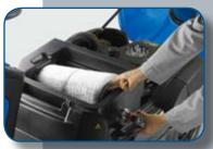
Filter can be removed and cleaned without tools. Polyester filter can also be washed, dried and reused.
