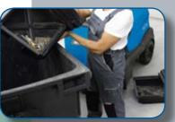
Large volume debris capacity is broken up into two easy-to-dump hoppers.
